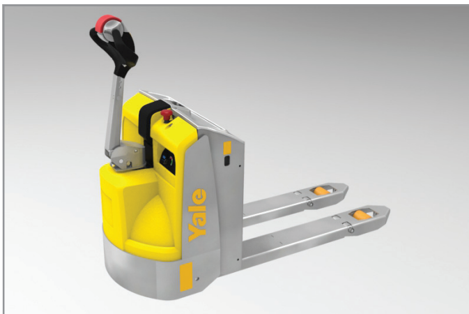
MP Series with hot zinc coated frame is more resistant to corrosion.
