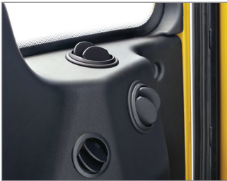
Insulated door with added ventilation for mist free view.
