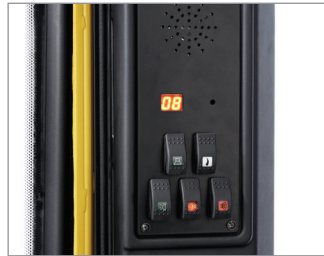
Cab heaters and controls.
